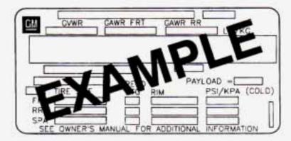
The Certification/Tire label is found on the rear edge of the driver's door. The label shows the size of your original tires and the inflation pressures needed to obtain the gross weight capacity of your vehicle.
